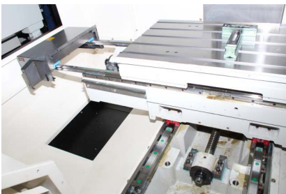
Increased inclination of base chute eliminate need of flush coolant
